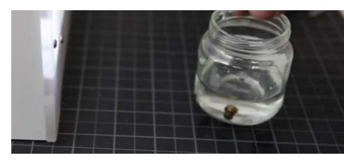
If your nozzle is still clogged after trying the above procedures, there is one more thing you can do. That is, assuming you've been printing with ABS. Remove the nozzle from the print head, put it in acetone, and leave it there for a few hours. The acetone will melt the material in the nozzle and enable it to be cleared with a needle.
